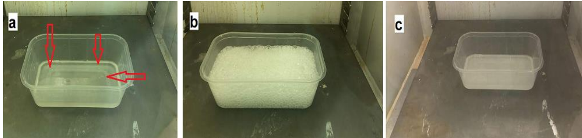
Figure 3-6 a) Mixture of the PU and isocyanate after stirring, b) in the vacuum degassing chamber, c) after degassing process.
