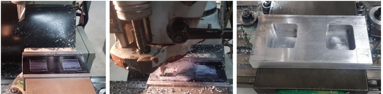
Figure 4-19 Manufacturing of the mould for casting the resilience test specimens.
