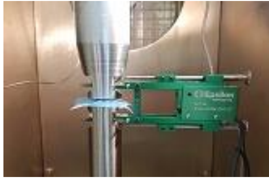
Figure 3-58 Universal test machine with special compression test fixture.
