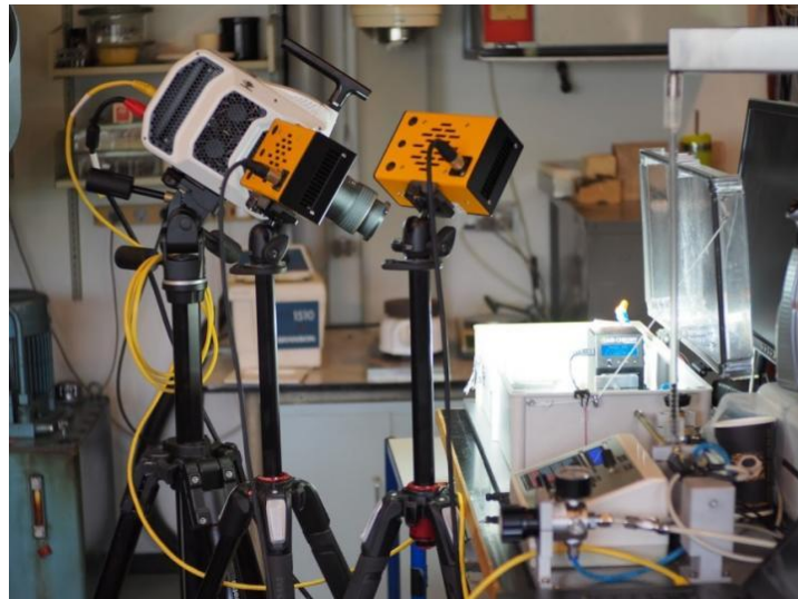
Figure 5-3. High speed camera (Phantom v2512 fast) for filming the ball impacts at 380,000 fps [161].
