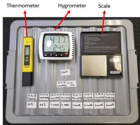
Figure 3-20 Measuring the environmental parameter that could affect the experiment.
