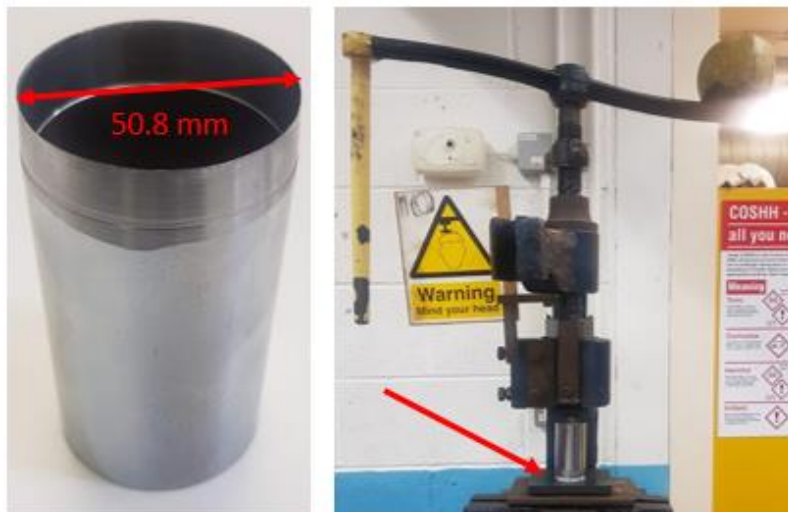
Figure 3-16 Manufacturing specimens for the water absorption tests.
