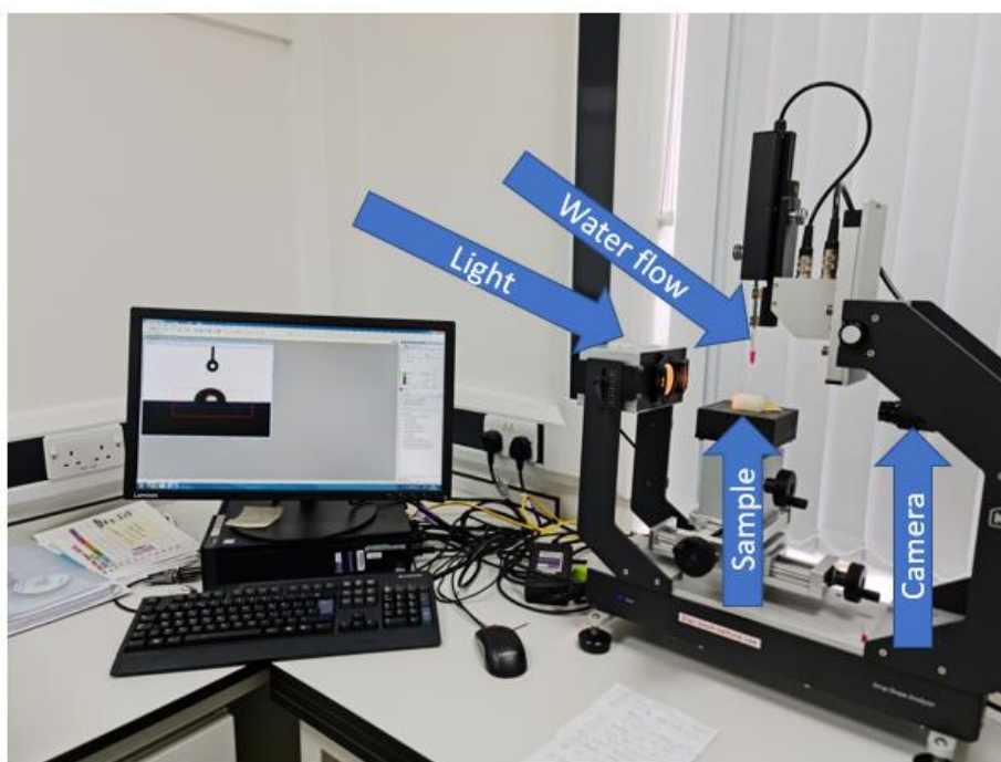
Figure 3-5 DSA30 contact angle measurement device.
