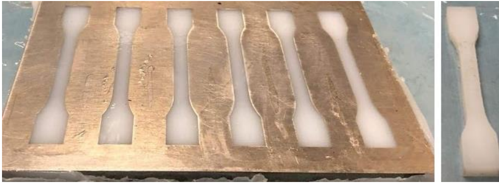
Figure 3-8 Casting of tensile test pure polyurethane specimens.
