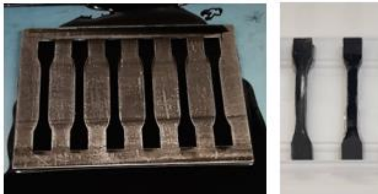
Figure 3-18 Manufacturing the tensile test samples.
