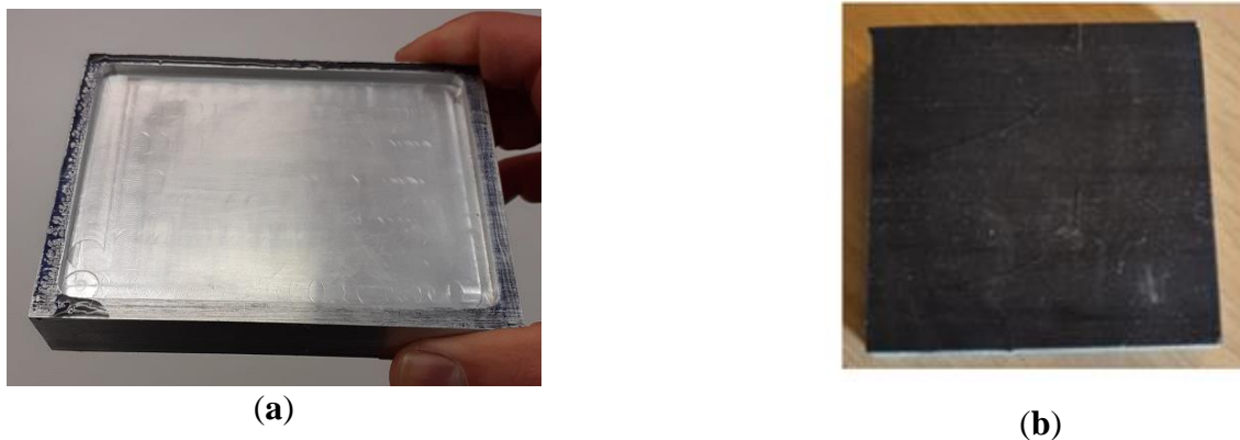
Figure 5-2. (a) Aluminium mould for casting thin coating film; (b) A finished rain erosion specimen with PU + GNP top coat.
