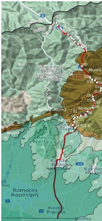
Figure 1: Vertical Road axis under study. The relevant geologic formation codes are depicted whereas the white dots indicate the cut slopes for which seismic risk has been undertaken.
