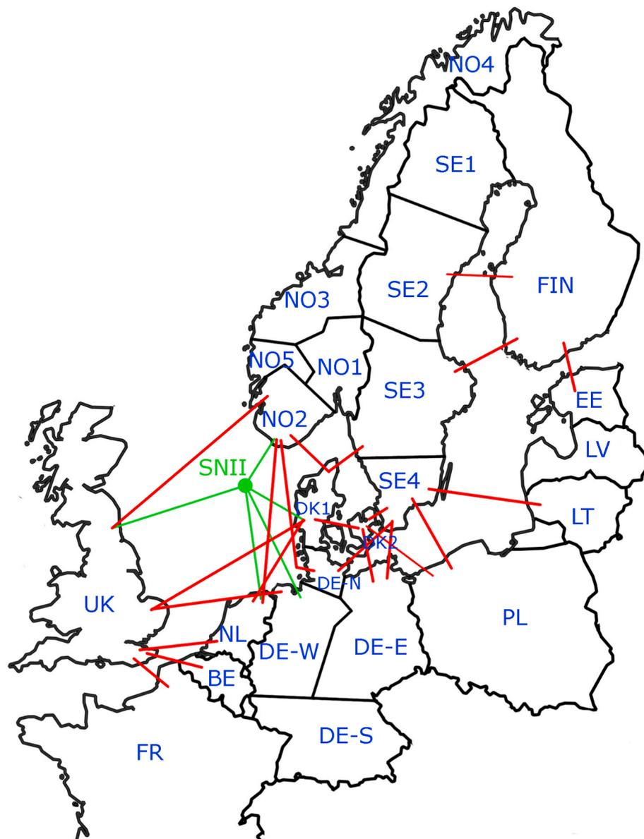
Fig. 1. Regional coverage of Balmorel with offshore interconnectors. Power lines to Søndre Norsjøen II (SNII) field are only included in the last approach.
