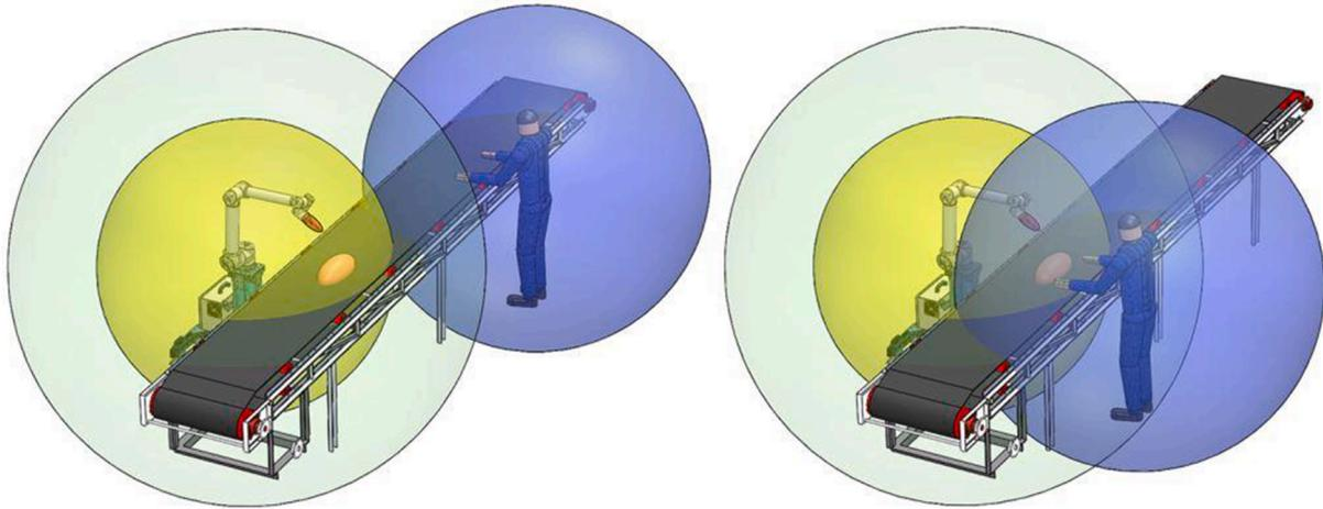
**Fig. 6.** Operational spaces for coexistence (left) and collaboration (right). Red: area of a tool, green: robot's operating space, yellow: collaborative workspace, blue: operator workspace.
