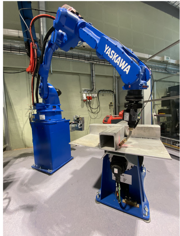
Fig. 9 The robot cell comprising a Yaskawa Motoman GP25 robot manipulator and a MT1-500 workpiece positioner
