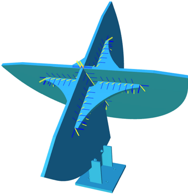
Fig. 5 Visualisation of wall vectors (blue) and initial approach vectors (yellow) automatically scanned and generated from CAD
