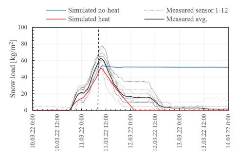
Fig. 3. Measured and simulated snow load during a snow fall event in Porsgrunn, Norway. The vertical dashed line signifies when power was applied to the modules.
