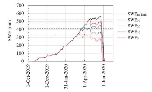
Fig. 5. Single year simulation of SWE for different return period melting limits (subscript in legend) in Tromsø the winter of 2019–2020. The horizontal dashed lines signify the SWE threshold for when power is applied.
