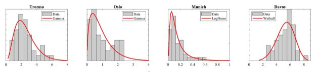
Fig. 4. Histogram of maximum annual snow load in kN/m<sup>2</sup> with the best fitting distribution for the four investigated locations.
