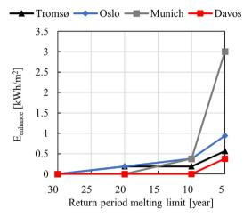
**Fig. 8.** The yield enhancement ( $E_{enhance}$ ) per year from the decrease in snow losses for different return period melting limits in relation to a PV system without snow mitigation (given in Table 3).
