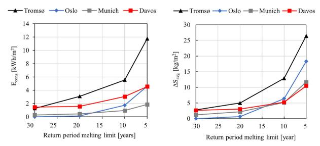
**Fig. 6.** a) Average annual energy consumption ( $E_{cons}$ ) and b) average annual snow load reduction amount ( $\Delta S_{avg}$ ) per year for a PV snow mitigation system with different return period melting limits.
