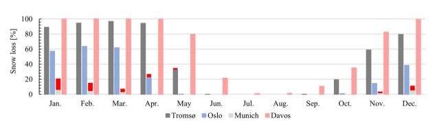
**Fig. 7.** Monthly snow loss [%] obtained from the energy balance snow model. The difference in snow loss between the 5-year return period melting limit and no melting limit is illustrated by the red bars. (For interpretation of the references to colour in this figure legend, the reader is referred to the web version of this article.)
