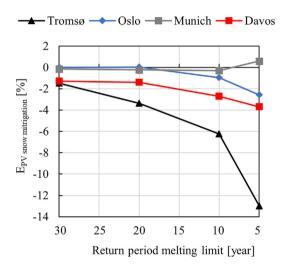
Fig. 9. Simulated influence of actively mitigating snow  $(E_{PV \ snow \ mitigation})$  for varying return period melting limits for the four locations.
