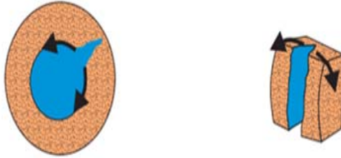
Figure 3 Tensile failure around boreholes (see online version for colours)
