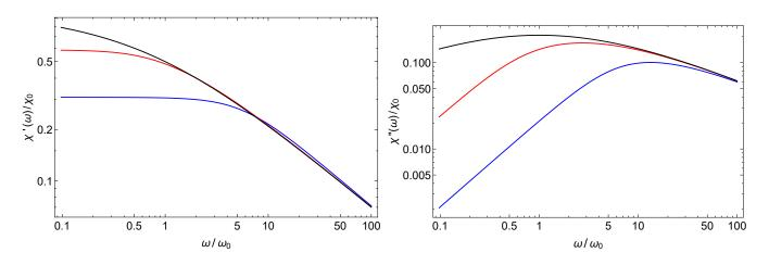
**Figure 7.** Behaviour of the complex susceptibility (log–log plot) for Cole–Cole relaxation with resetting. The black lines correspond to Debye relaxation without resetting, while the red and blue lines correspond to *r*-parameter values of 0.5 and 5, respectively. The parameter  $\alpha = 0.5$ . **Left panel**: real part. **Right panel**: imaginary part (dielectric loss).
