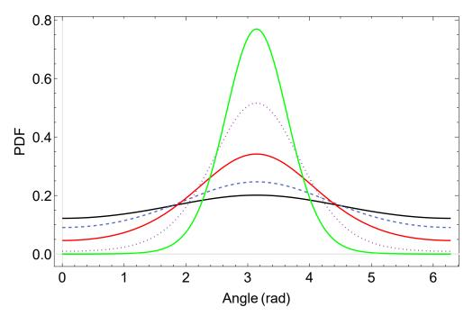
**Figure 2.** Probability density function (PDF) given by Equation (2) at different ratios  $\mu E/kT$ . The black line corresponds to  $\mu E/kT = 0.25$ , the dashed line corresponds to  $\mu E/kT = 0.5$ , the red line corresponds to  $\mu E/kT = 1$ , the dotted line corresponds to  $\mu E/kT = 2$ , and the green line represents the case  $\mu E/kT = 4$ .
