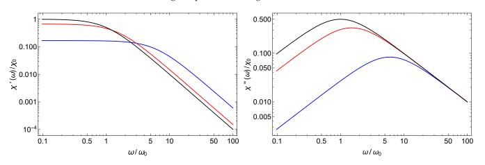
**Figure 5.** Behaviour of the complex susceptibility (log–log plot) for Debye relaxation with resetting. The black line corresponds to Debye relaxation without resetting, while the red and blue lines correspond to *r*-parameter values of 0.5 and 5, respectively. **Left panel**: real part. **Right panel**: imaginary part (dielectric loss).
