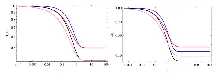
**Figure 10.** Behaviour of the correlation function (80) for the Havriliak–Negami relaxation in the presence of resetting. The parameters are taken as follows:  $\lambda_1 = 1$ ,  $\tau = 1$ , and  $\alpha = \nu = 1$  (Debye relaxation with resetting, blue line),  $\alpha = 3/4$ ,  $\nu = 1$  (red line),  $\alpha = 1$ ,  $\nu = 3/4$  (black line),  $\alpha = \nu = 3/4$  (pink line). **Left panel**: r = 1; **Right panel**: r = 0.5.
