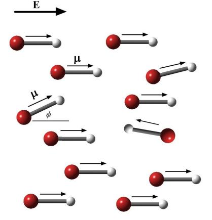
Figure 1. A system of dipoles subjected to external uniform electric field with a magnitude *E*.
