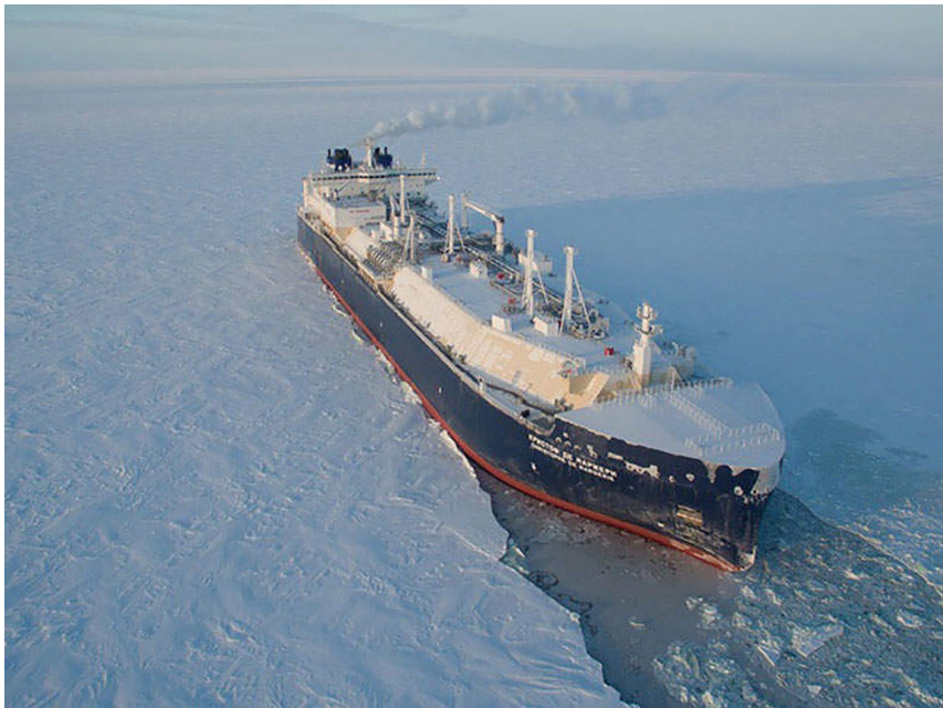
Figure 14.5 Double Acting Tanker. The Christophe de Margerie-class ice-breaking LNG carriers are built by DSME (Daewo Shipbuilding Marine Engineering) for the Yamal LNG project. Image courtesy of Dmitrii Lobusov.
