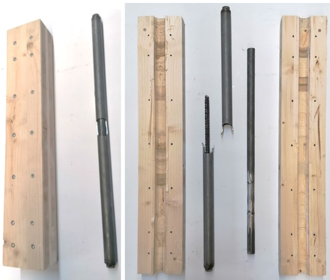
Fig. 15 Intact and broken hold-down specimens with timber casing
