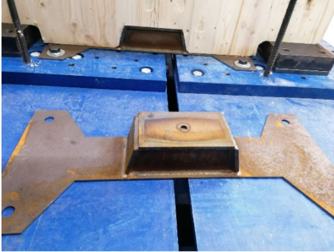
Fig. 23 Photos of the steel shoe for base shear fixing of the CLT shear walls
