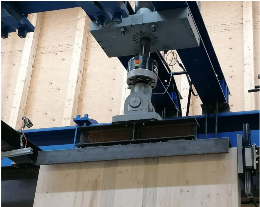
Fig. 25 Vertical constant loading system
