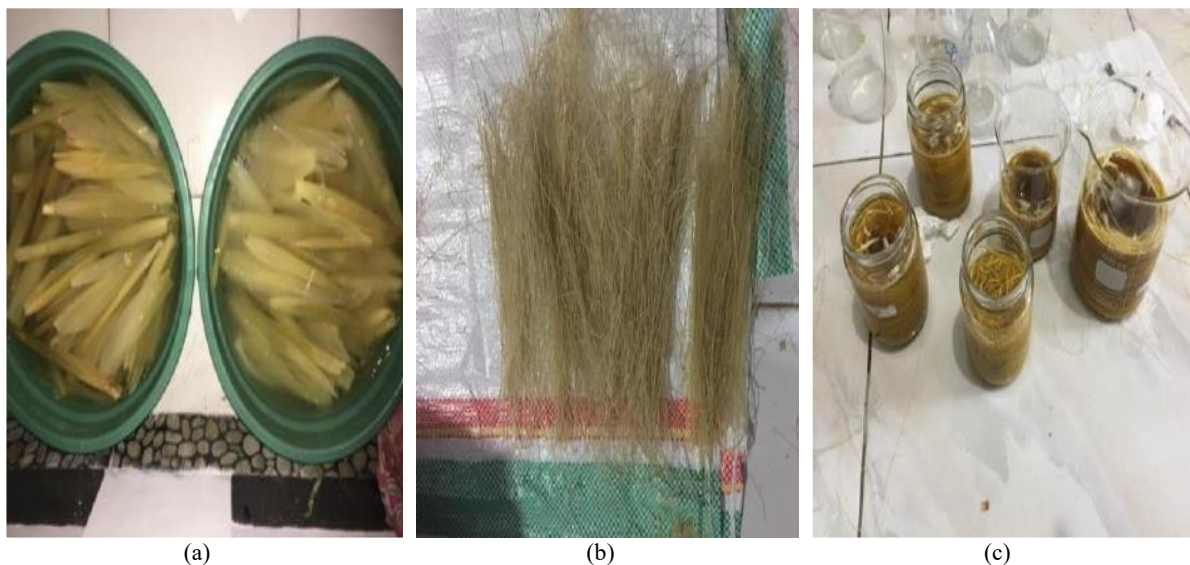
Figure 1. (a) Corn husk soak for 10 days, (b) corn husk combing, and (c) corn husk treated with NaOH concentration of 5%.
