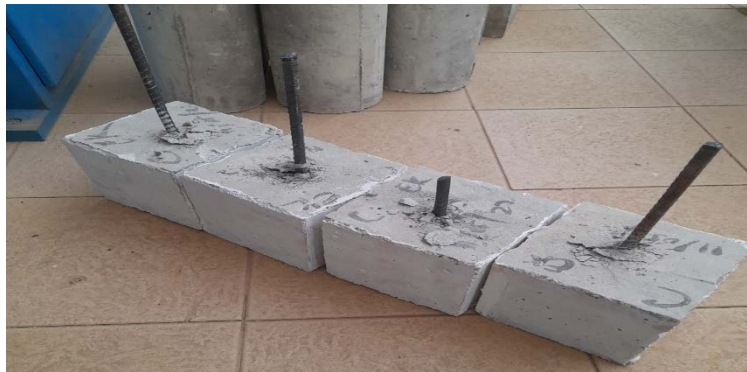
Fig. 9. Rebar pullout bond failure of specimen with 10 mm steel rebar.
