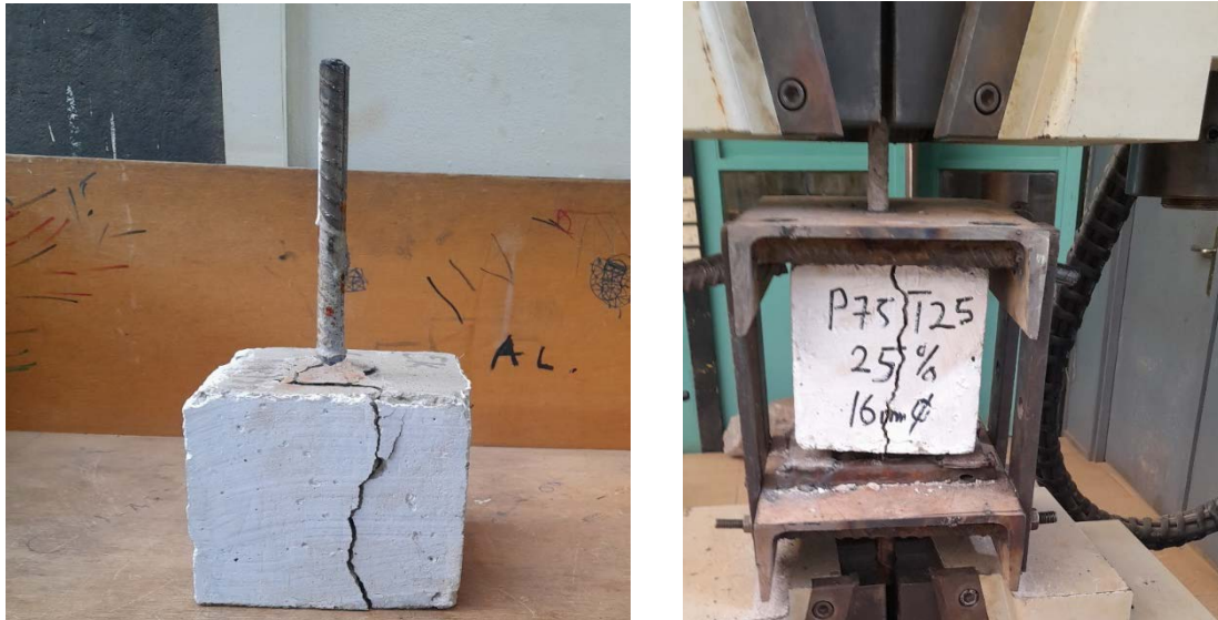
Fig. 8. Tensile splitting or crushing of specimen with 16 mm diameter deformed mild steel rebar
