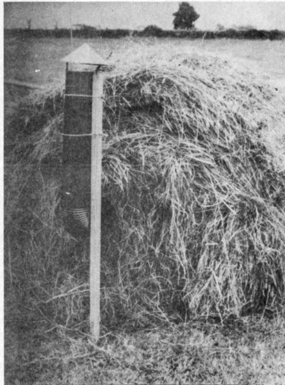
Figure 22. Typical Chimney Placement During Drying Test.
