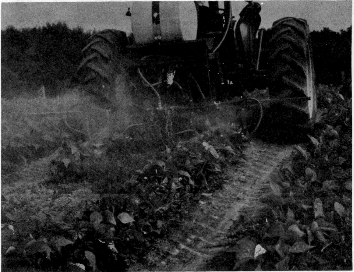
Figure 1. Medium-volume, two-row hydraulic sprayer used in the application of the fungicide solution and fluorescent particle suspension.
