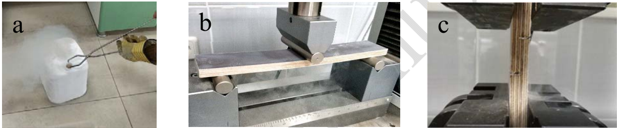
110 Figure 1: Freezing treatment of plywood samples (a), bending test (b), tensile-shear test (c).
