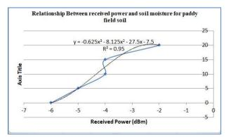
**Fig. 12:** Relationship Between received power and soil moisture for Paddy field soil
