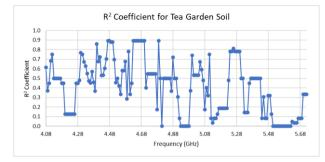
**Fig. 5:** Relation between frequency and R<sup>2</sup> Coefficient for Tea Garden Soil
