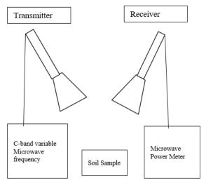
Fig. 2: Schematic Representation of the Experimental Set-up
