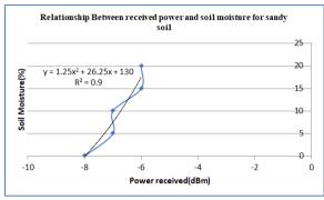
Fig. 8: Relationship Between received power and soil moisture for Sandy Soil
