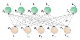
Figure 2: The basic unit of an Boltzman machine
