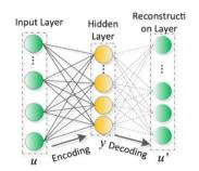
Figure 1: The basic unit of an auto-encoder
