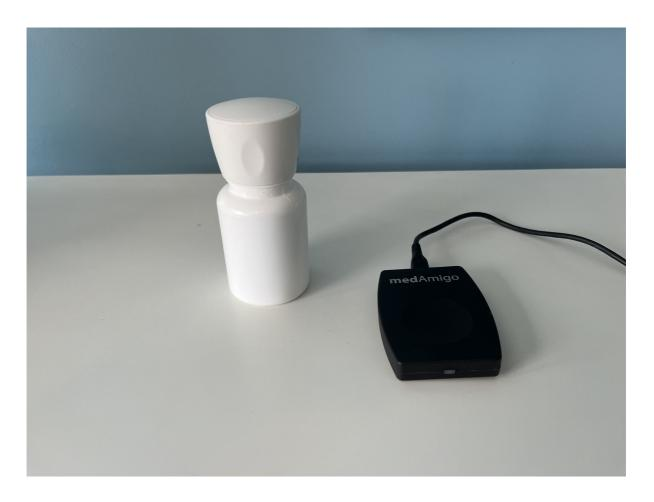
**Figure 1.** The medication Adherence Monitoring System (MEMS), consisted of an electronic cap, medication container, and a reader, enabling the programing of the device as well as transferring the adherence data
