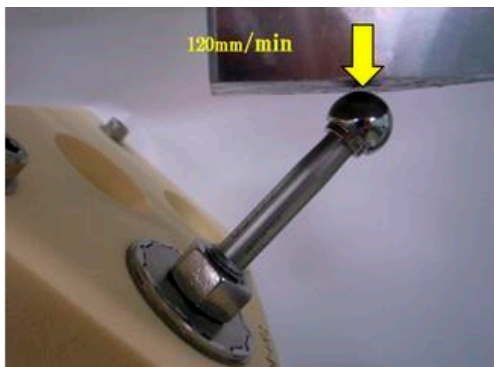
Fig. 3B. Close up photo of lever-out test apparatus
