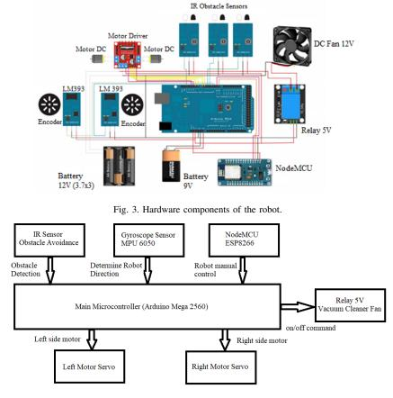
Fig. 4. Hardware block diagram.
