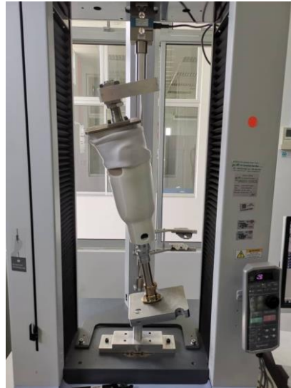
Figure 4. Experimental set-up of lower limb prosthetic leg structural test.
