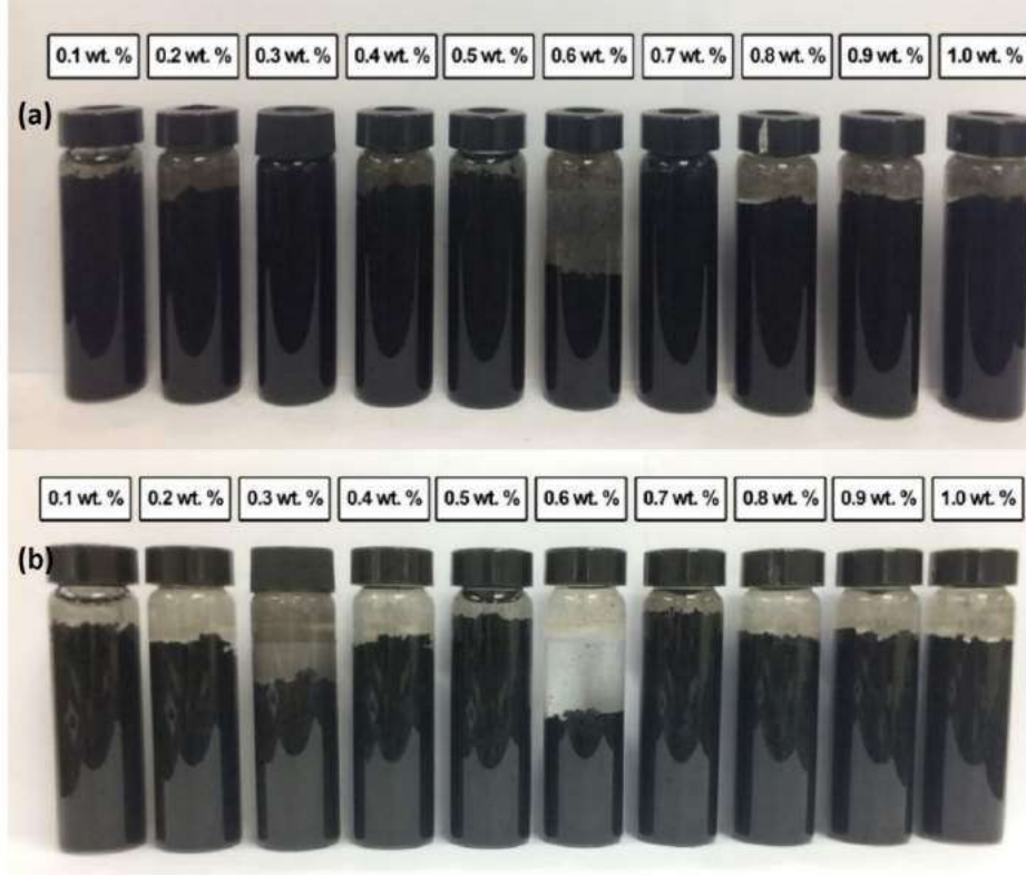
Figure 5. Stability and dispersion condition of various weight percentages of the commercial MWCNTs based nanofluid with a surfactant of PVP. (a) 0.1 wt.% to 1.0 wt.% showing stable dispersion. (b) 0.1 wt.% to 1.0 wt.% showing sedimentation.
