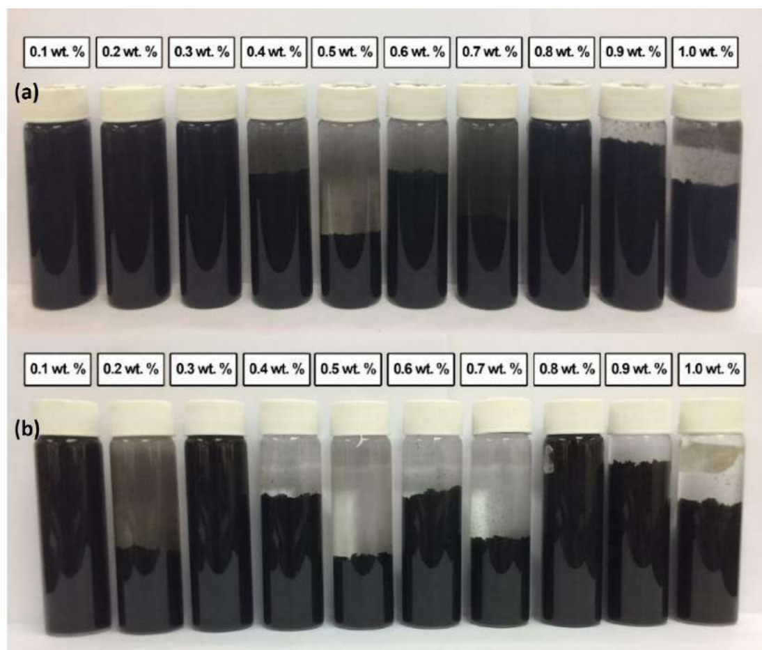
Figure 6. Stability and dispersion condition weight percentage of the commercial MWCNTs based nanofluid with surfactant of PVP for (a) 0.5 h; (b) 100 h after homogenization and sonication process.
