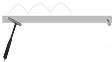
Fig. 2. The roving hammer test.
