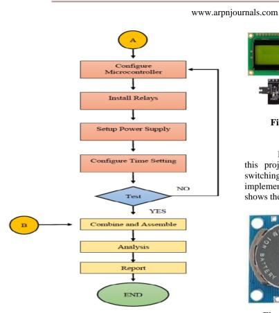
Figure-2. Flow chart for configuring the switching system.
