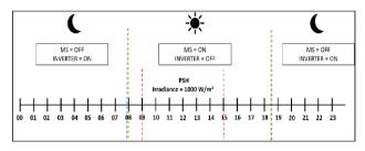
**Figure-10.** Timeline to guide user in controlling the switching timing for manual mode.
