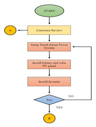
Figure-1. Flow chart for installing the stand-alone PV system.
