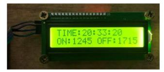
Figure-9. Configuring "ON" and "OFF" value of manual mode.
