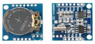
Figure-5. Real-Time Clock (RTC) 1307 module.
