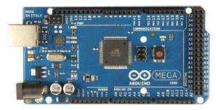
Figure-3. Arduino mega 2560 R3 board.
