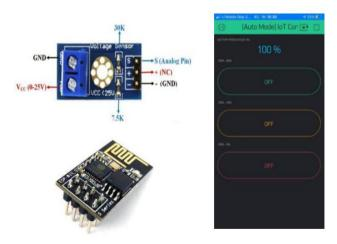
Figure-6. Voltage sensor, ESP8266 Wi-Fi module.
