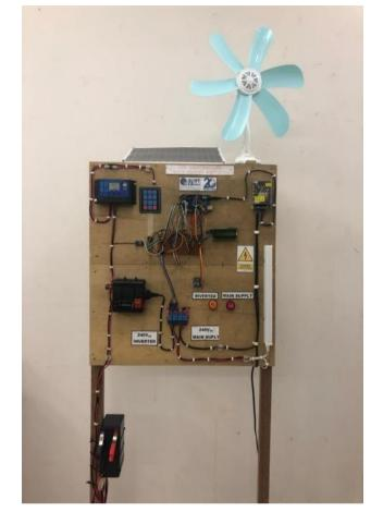
Figure-8. Hardware development of IoT controlled hybrid power switching.
