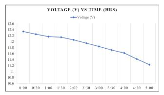
Figure-12. Depletion of battery voltage capacity against discharge time in hours.
