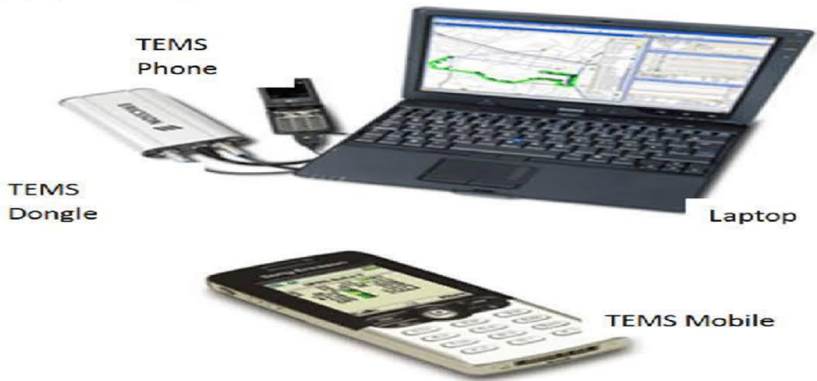
Figure1: TEMS Measurement Tool used for Field gathering of RSSI Data.
