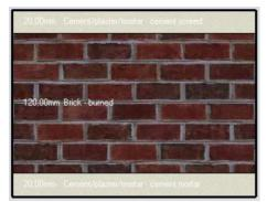
Figure 3. Composition of the layers of non-structural walls.
