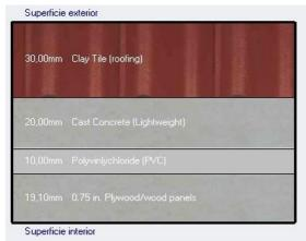
Figure 5. Current state of the roof of the house case study and its design of the composition
