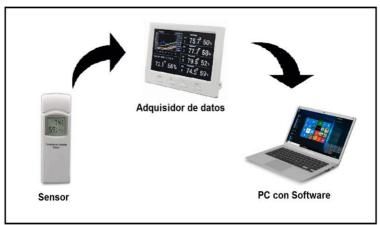
Figure 6. Diagram of the Hygrothermal monitoring system
