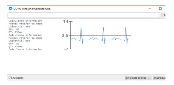
Figure 10. Monitor serie and ECG fixed and filtered in MATLAB
