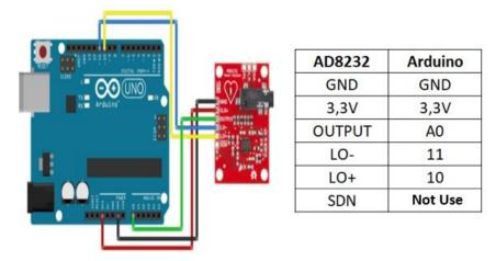
Figure 4. Connection between Arduino and AD8232 Sensor
