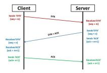
Figure 1. An illustration of the TCP three-way handshake
