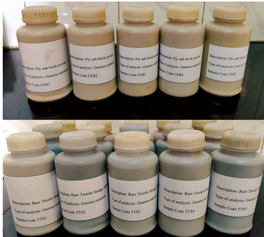
Fig. 2 — Packed and Sealed containers under Equilibrium condition.
