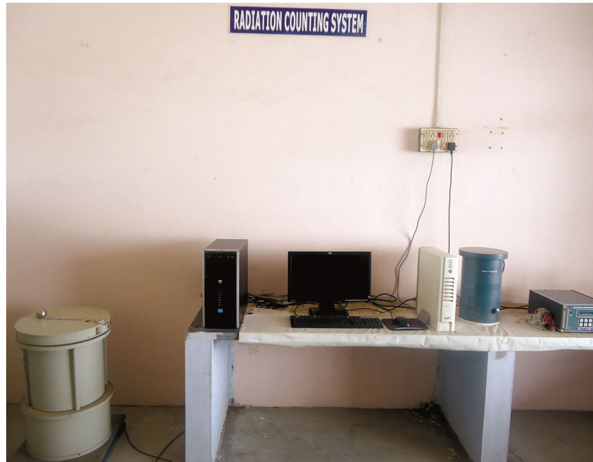
Fig. 3 — Radiation Counting system with NaI detector.
