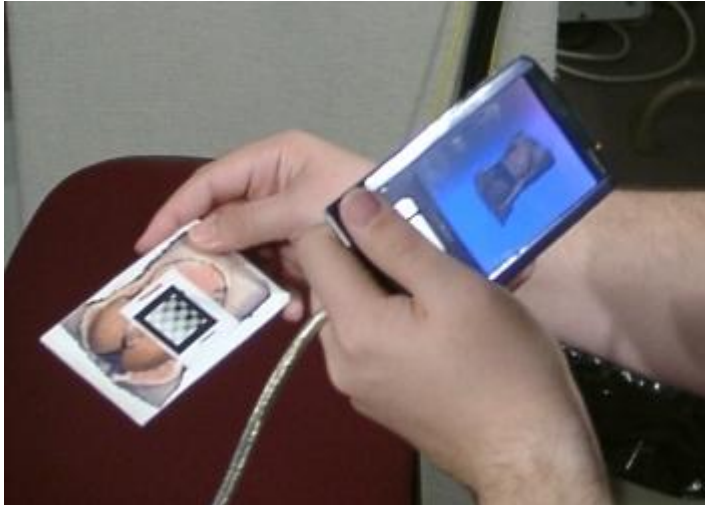
Fig. 2. Handheld prototype. The prototype uses a PointGrey DragonFly [23] camera mounted on the PDA (in the left hand). The prop (in the right hand) has a printed image of our training torso on it, along with a grayscale pattern. We use ARToolkit [24] to track the surrogate with respect to the PDA (remote.)
