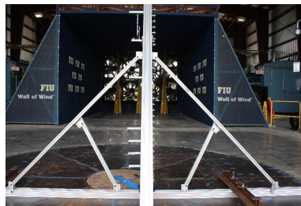
Figure 8. Instrumentation for profiles of wind velocity.
