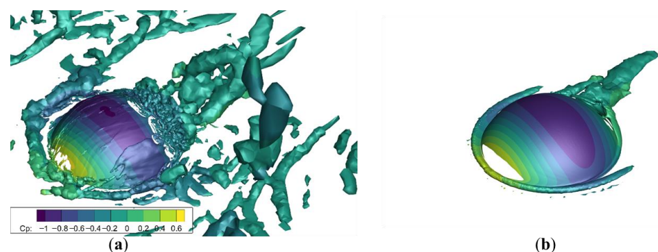
Figure 27. Iso-surfaces of Q criterion ( Q = 2000 ) colored by mean pressure coefficients: (a) LES; (b) SST k-\omega .
