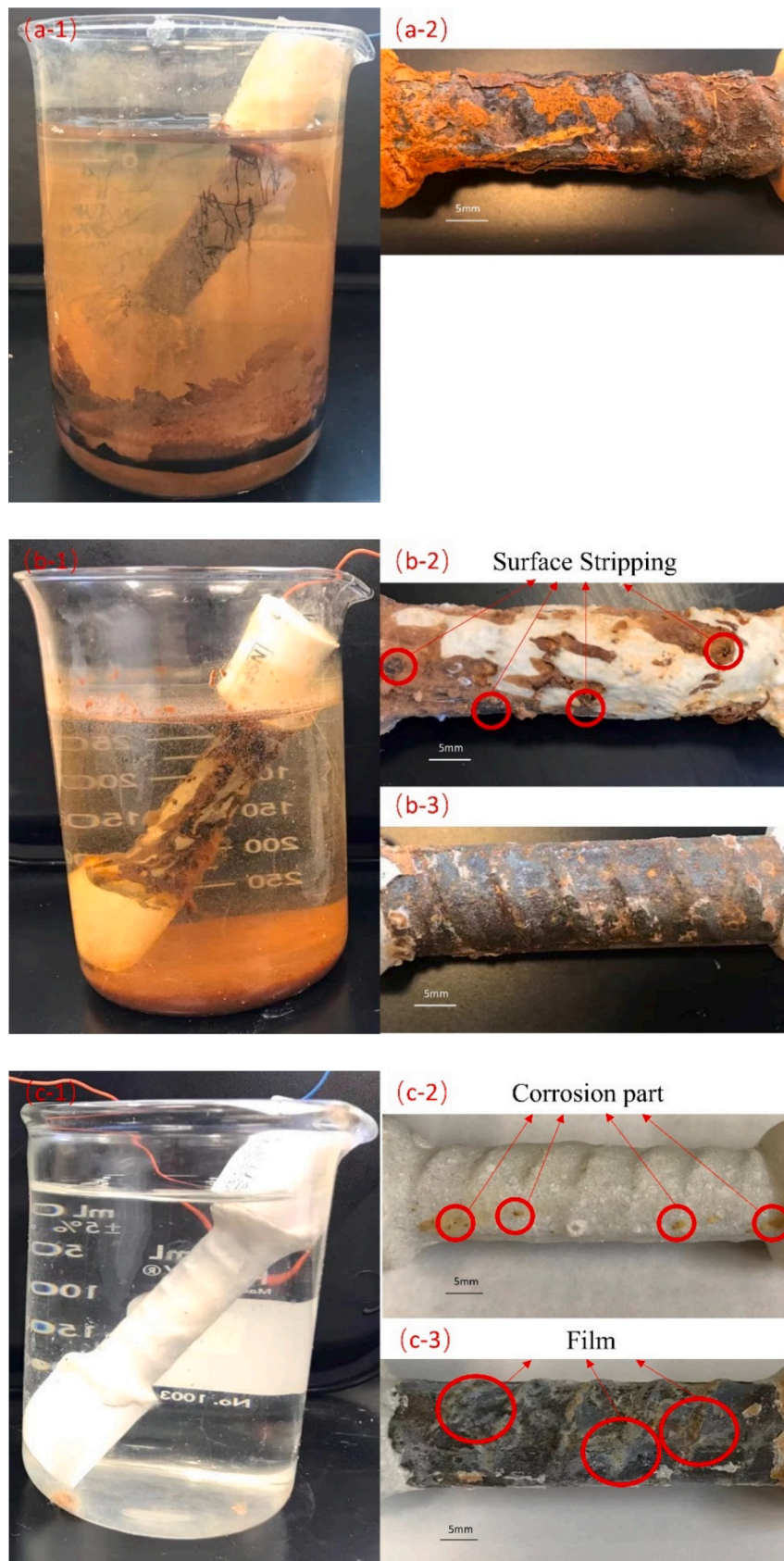
Fig. 12. Bar surface conditions (number1: test condition, number2: samples without any treatment and number 3: samples with peeling off the coating) of samples after 5376 h EC test for:(a) UN, (b) OPC and (c) MKPC.
