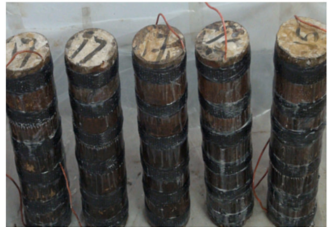
Fig. 3. CFRP partially wrapped columns before freeze–thaw erosion.
