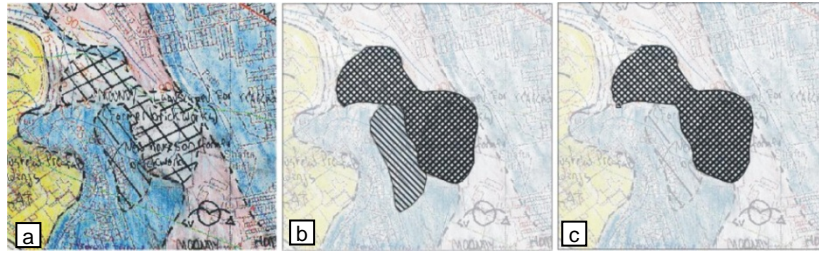
Figure 9. Example showing how appropriate visualisation and processing identifies areas of infilled ground without loss of primary attribution (not to scale):
