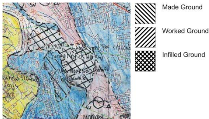
Figure 6 Example showing the traditional representation of Artificial Ground on a 1:10,000 scale fieldslip (not to scale). Digital compilation using the current classification can result in the loss of relevant information.
