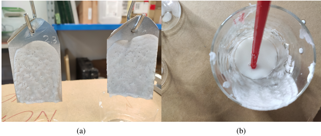
Fig. 3.18 (a) Aluminium testing plate with coated surface, (b) mixture in progress
