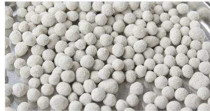
Fig. 3.6 Activated alumina pellets
