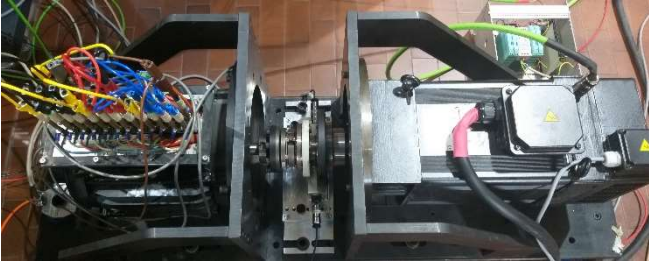
Fig. 4. View of the IM under test (left), torque transducer (middle), and driving machine (right).
