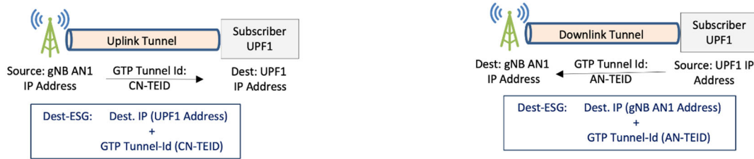
Figure 5: Example Diagram of Endpoint Security Group Derivation
