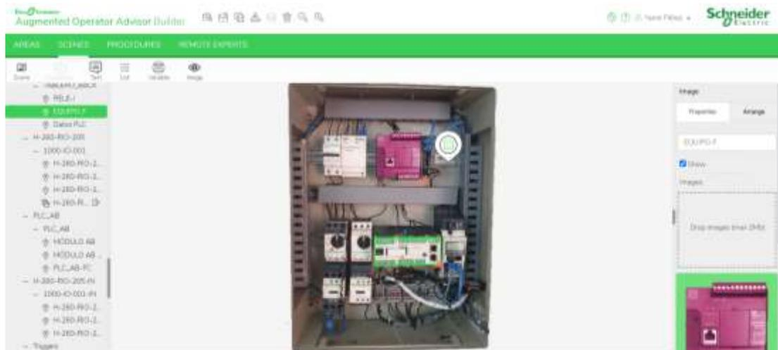
Figura 4 Vista del entorno del software EcoStruxure Augmented Operator Advisor.
