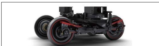
Ilustración 13 Bogie efWING (environmentally friendly weight-saving innovative new generation truck) Fuente:(Kahnert, 2015)
