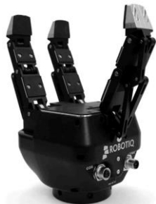
Fig. 8 The Robotiq 3-Finger adaptive gripper that's used in industry.
