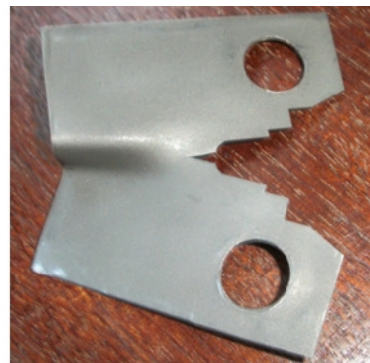
Fig.3. Determination of the crack propagation from FE Analysis
