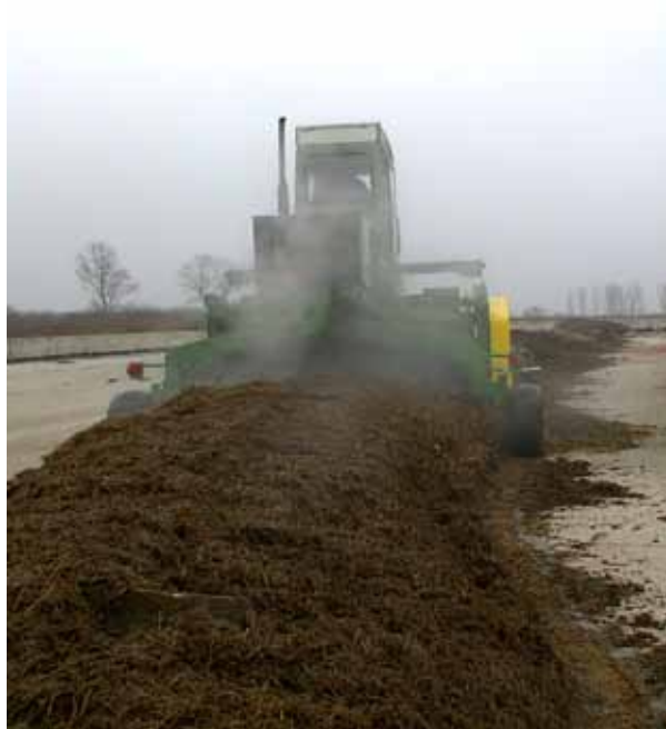
Slika 1. Mašina za negu stajnjaka u radu i formirana prizma Figure 1. Machine for manure treatment in action and formed prisms
