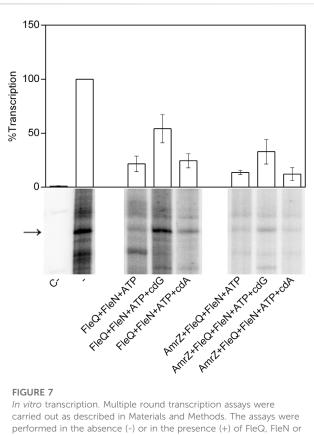
performed in the absence (-) or in the presence (+) of FleQ, FleN or AmrZ. When indicated, ATP, c-di-GMP or c-di-AMP were also added to the reaction. C- indicates a reaction without template DNA. The 232 nucleotide mRNA synthesized from P<sub>wssA</sub> is point out by an arrowhead. The graph shows the average amount of the mRNA produced as percentage of the condition without any protein (-). Error bars correspond to the standard deviation of six different transcription assays.
