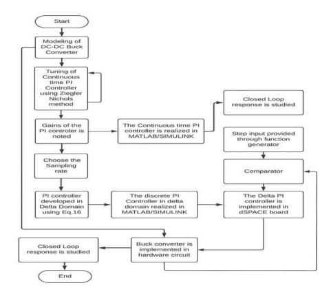
Fig. 5 Flowchart describing the complete mechanism of controller design in the delta domain
