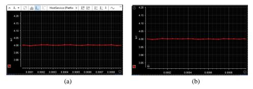
Fig. 13 Regulation of output voltage for load resistance of (a) 100  $\Omega$  (b) for 100 k $\Omega$
