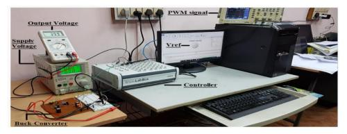
Fig. 12 Complete hardware setup with 4 volts as reference
