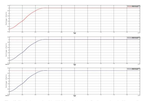
Fig. 10 Simulation result with 100 kΩ resistance (a) Continuous domain PI controller response, (b) Delta domain PI controller response with a sample rate of 0.5 sec, (c) Delta domain PI controller response with a sample rate of 0.00001 sec
