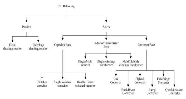
Figure 2. Active balancing types
