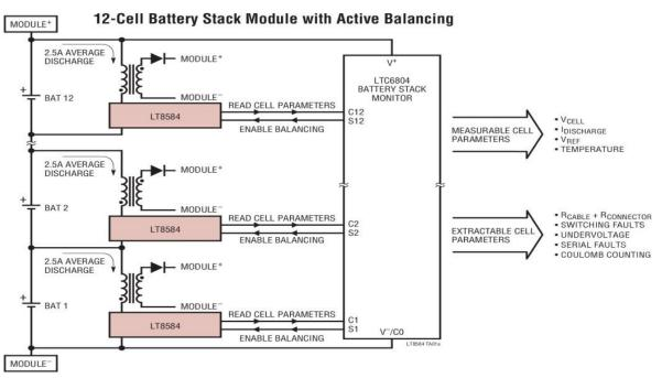
Figure 1. Modern active balancing unit
