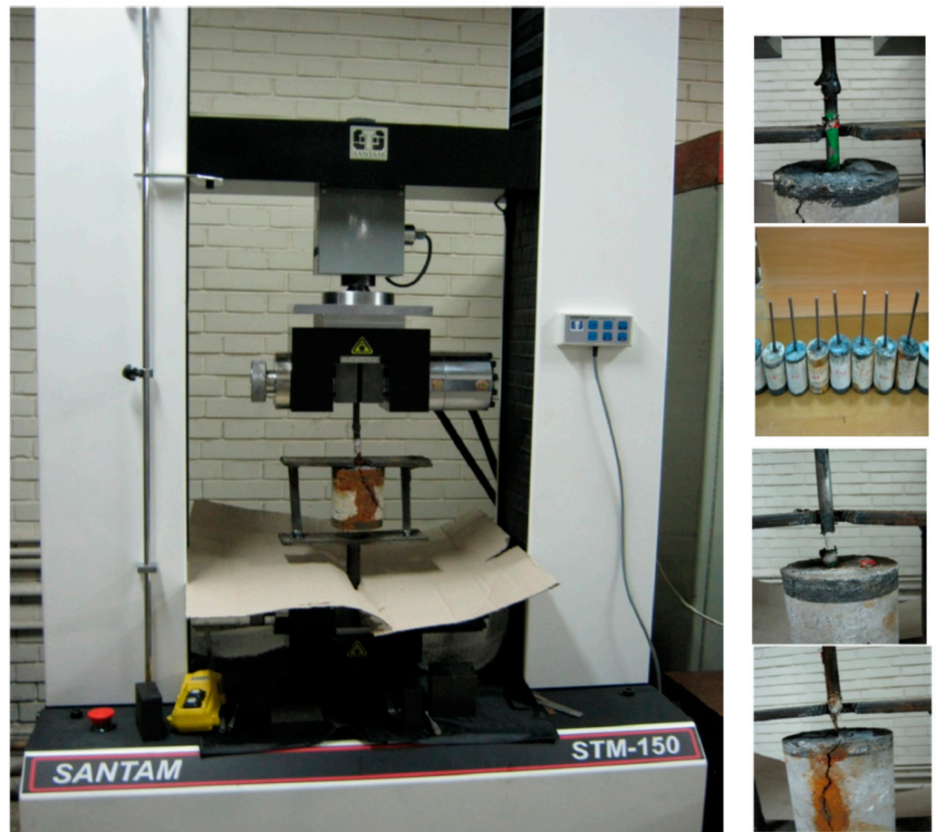
Figure 2. Pullout of steel–concrete bond joints test apparatus.
