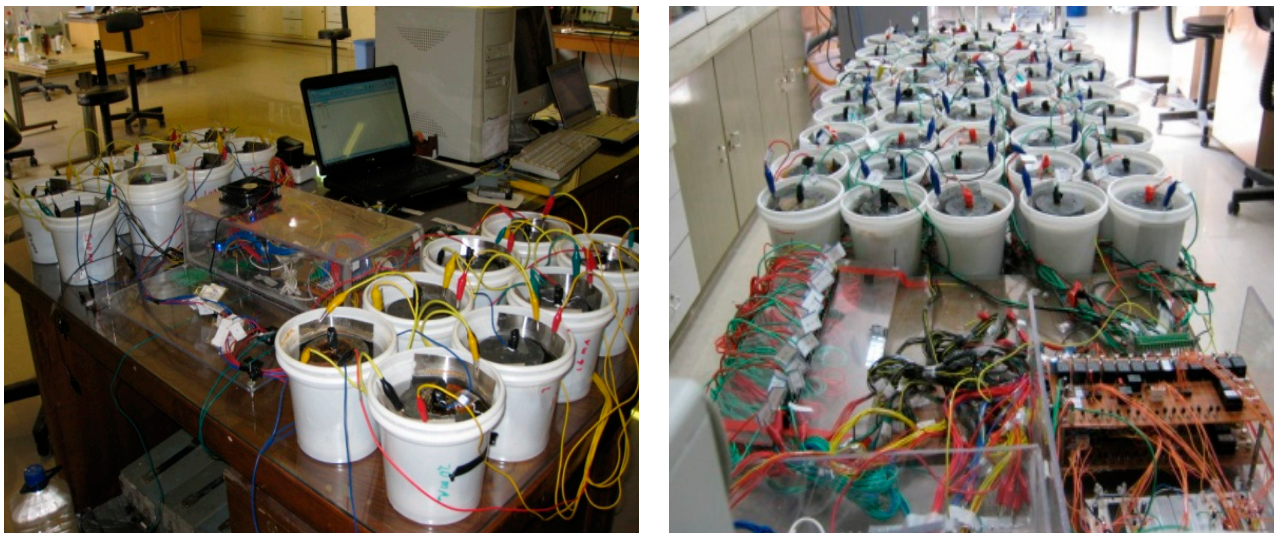
Figure 1. The accelerated corrosion test which measured and displayed data in a corrosion measuring device.
