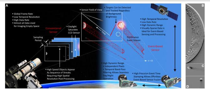
FIGURE 1 | Comparison between conventional imaging (A), event-based vision for space imaging, and SSA tasks. Sub-figures show the event-based output of the Moon (B), Saturn (C), and Jupiter (D) through a telescope. Figure from Afshar et al. (2020).
