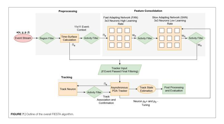
The FIESTA algorithm was written in C++, using the Eigen and OpenCV library. The asynchronous PDA tracking code was built onto a basic GNN tracking and Kalman filter framework (Konstantinova et al., 2003). All results were obtained using a PC with an Intel Core i7-7700HQ CPU @ 2.80 GHz  $\times$  8 with 16 GB of RAM. The PDA algorithm weight calculations were conducted in the log space.
