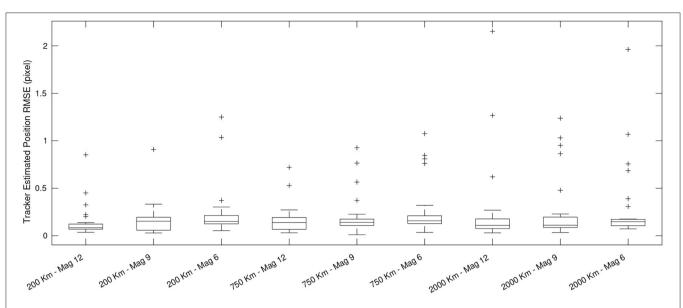
FIGURE 13 | Comparison of the RMSE localization error (pixel) recorded in each of the nine simulated RSO altitude and magnitude brightness scenarios. In each scenario, 30 different recordings were evaluated.
