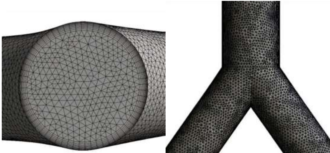
Figure 4.2. Computational mesh for the section of G4 (a) Refined inflation mesh near the airway wall (b) The mesh resolution on the airway wall.
