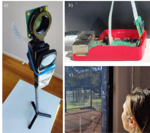
Figure 9. DGP field measurement: (a) HDR camera; (b) False-color imaging; and (c) Human subjects' assessment.
