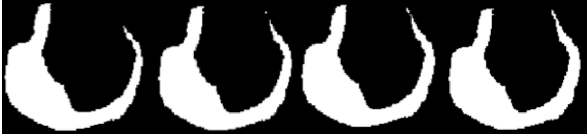
Figure B-2 Sample diagram showing the iterative process to achieve suitable shell image by the thickening of the anterior portion
